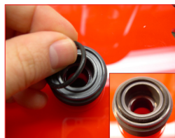
1.) Seat the 1 st o-ring in position
